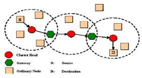
Fig. 1. Architecture of Mobile ad hoc network.
